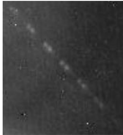
Figure 7. The dispersion effect: higher orders separate into double dots because the filter passes two major wavelengths, Fe IX at 171.073 \text{ \AA} and Fe X at 174.507 \text{ \AA} , and the longer wavelength is diffracted more than the shorter one. This picture is magnified and brightened from the box in Figure 1.
